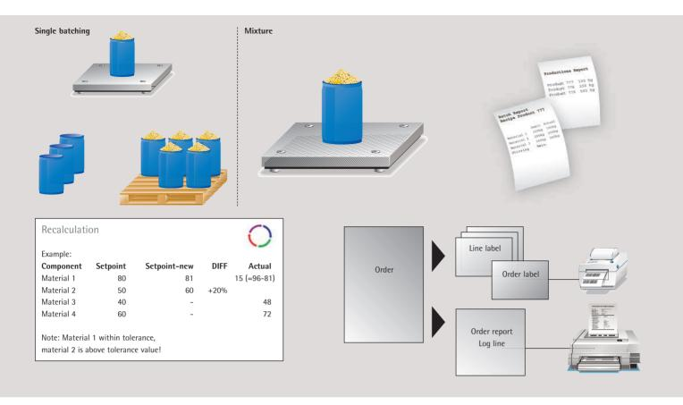
Manual batching is supported by a bargraph display. When the operator has confirmed the end of batching, the tolerance check is carried out and subsequently the label and corresponding report line are printed. Labels can be configured directly in the equipment and can also be precisely adapted to the customer's requirements with the aid of an extra software tool.
