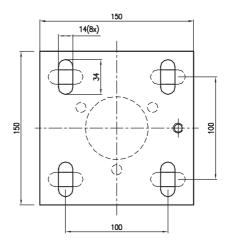
PR 6021/00N, Top and bottom load disc incl. rubber ring and earthing strap
