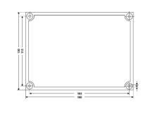
Power Supply: 85-250 V~, 50/60 Hz Electrical protection class: II Integrated Sensor Supply: 24 V =, 100 mA max. Power Consumption: 15 V<sub>A</sub> max. Depth, including transparent lid: 150 mm Operating Temperature Range: 0... +40° C Storage Temperature Range: -40... +85° C Ingress protection: IP 65
