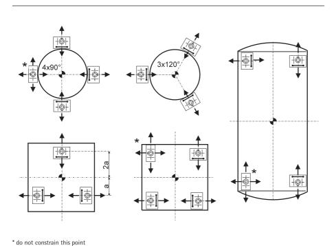
The range of PR6002 mounting kits has been specially designed for the PR6202 load cell family to guarantee best weighing performance and maximum suitability for hygienic environments. Capacities from 1t to 50t per load cell are available. The design follows the recommendations of EHEDG for hygienic design and consistently avoids gaps and undercuts. The surface quality is conform to international standards.
