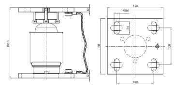
PR 6021/00N, Top and bottom load disc incl. rubber ring and earthing strap
